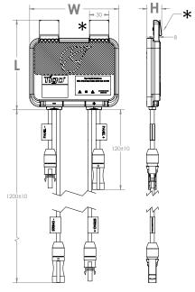
\*Clips can be removed for rack mounting
